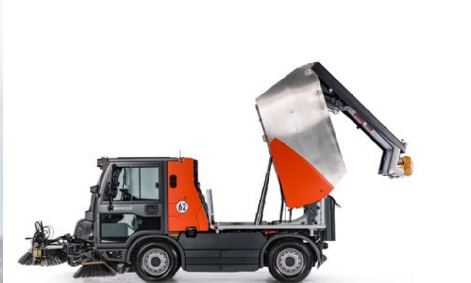
The smooth-surfaced stainless-steel hopper can be emptied quickly and easily and is particularly easy to clean.
