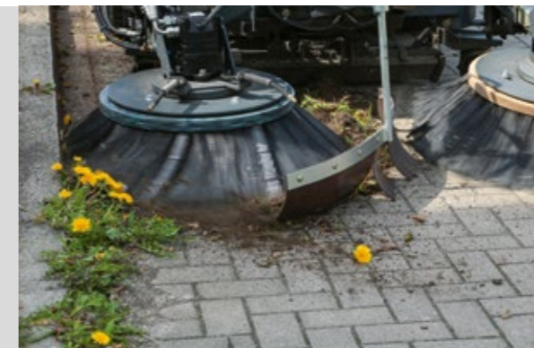
Chemical-free against weeds: with a weed broom for mechanical removal and collection.
