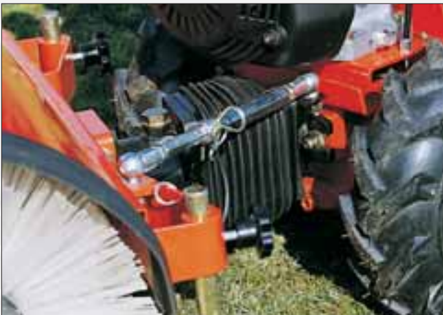
Quick and easy changing of the attached units by 2 screws. Equipment with robust p.t.o. shaft for efficient power transmission from gear to an implement such as e.g. the sweeper.
