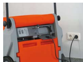
On-board battery charger to charge at any available plug socket.
