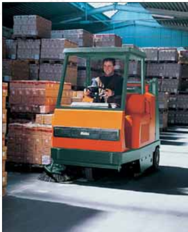
Cleanliness and safety: In the warehouse area safety is of the utmost importance. Here, for example, the overhead guard gives the operator additional protection.
