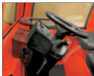
Adjustable steering column – relaxed driving position.
