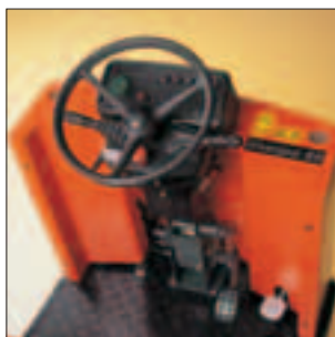
All operating elements are clearly laid out within direct view and reach of the operator. The swivelling steering wheel with sturdy steering as well as adjustable driver's seat guarantee the highest level of drive comfort.
