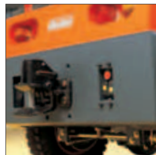
Heavy-duty Rockinger bolt coupling for towing loads up to 5 t. When attaching heavy transport vehicles, the reversing button proves to be especially handy. This makes it possible to guide the Hako Sherpa S5 on to the shaft from the rear.
