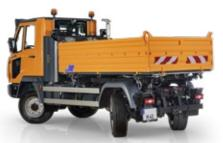
All-terrain: with all-wheel drive and continuously variable traction drive for optimum performance, optional all-wheel steering for easy manoeuvring and differential locks as standard for the right power distribution in demanding terrain.
