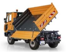
Unloading possible in any direction: large loading area with pendulum tailgate at the rear - ideal for transporting bulk goods or construction site work, for example.
