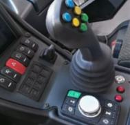
Joystick for intuitive, sensitive control of the most important functions, clearly arranged control panel with easy-to-reach buttons and colour multifunction display.
