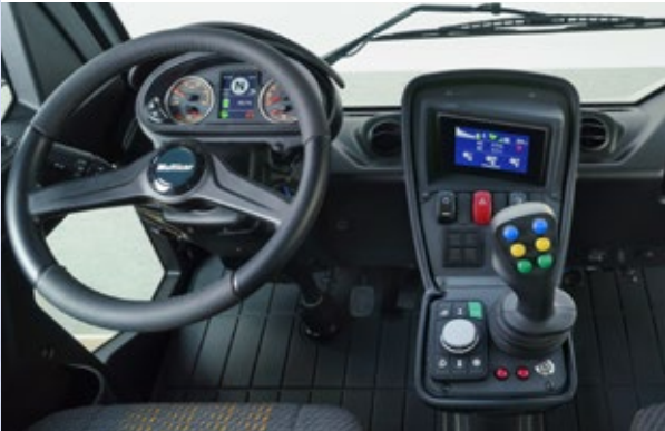
Everything at a glance, everything under control: joystick for intuitive control of the basic functions, clearly arranged control panel with easy-to-reach buttons and colour display for important information.
