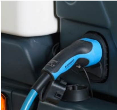
Fast, simple and safe charging: overnight with 22 kW AC or in between with up to 120 kW DC (fast charging).
