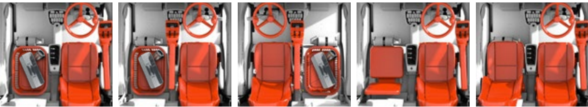
Made for the driver: different seat configurations – with or without storage compartments – not only provide variable utilisation options but also offer the driver significantly more space in the cab.
