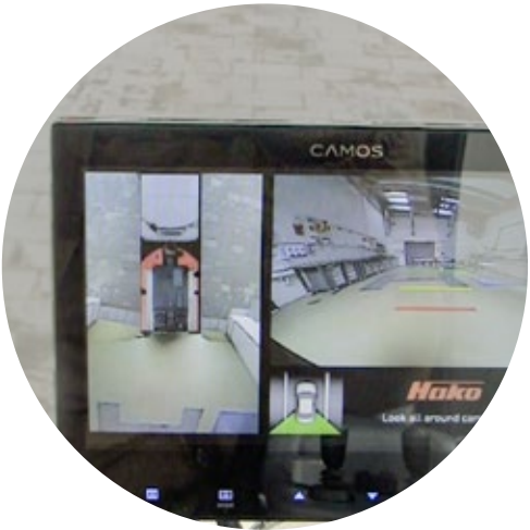
Safe: the camera system widens the driver's viewing angle by 270°.
