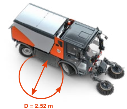
Great performance, small turning circle: thanks to its compact dimensions and all-wheel steering.
