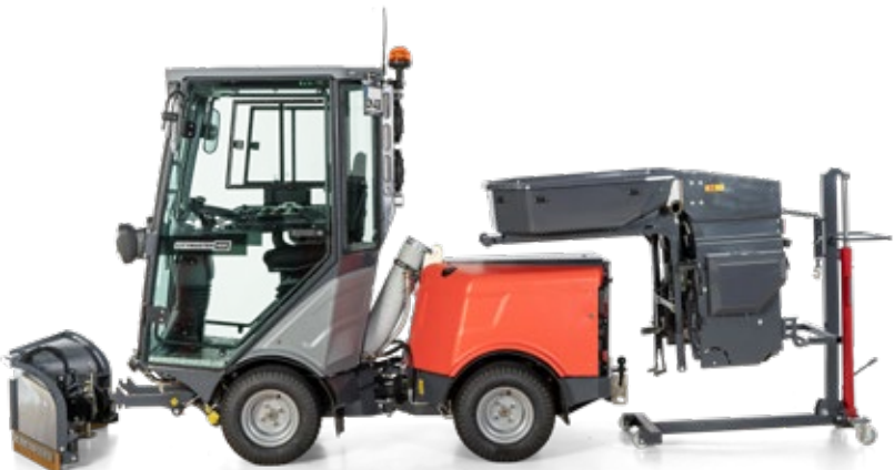
The quick-coupling triangle enables simple, tool-free and back-friendly implement changes. Rear attachments can also be changed by just one person thanks to unique quick couplings.
