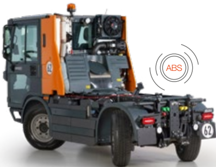
The machine has the excellent manoeuvrability of a lorry implement carrier – and gets you around every corner easily thanks to all-wheel steering.
