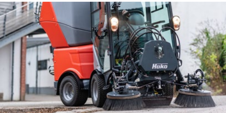
Clean sweeping: thanks to the hydraulically driven 2-broom sweeping unit and patented circulating water system.
