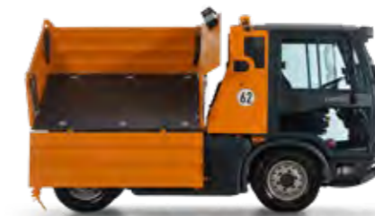
Side tipper for quick, controlled unloading – even in confined spaces.
