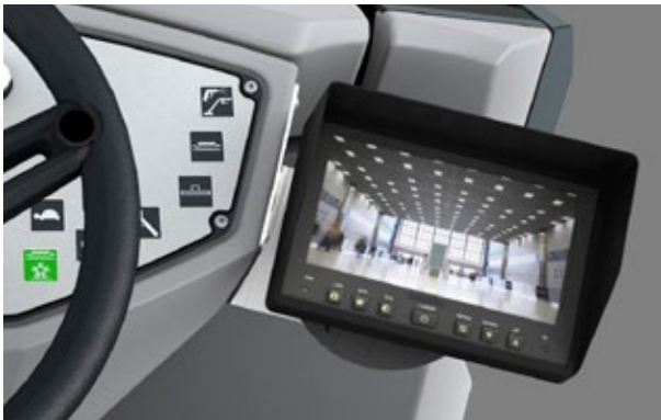
Rear-view camera When reversing, the optional rear-view camera and the monitor next to the control panel provide a better view to the rear.
