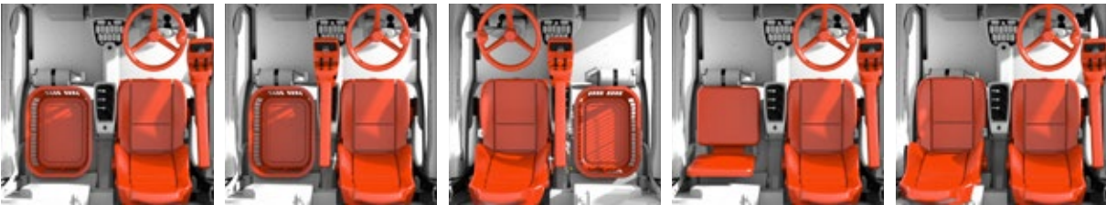
Made for the driver: Different seat configurations with comfort and auxiliary seat and with or without storage options not only allow variable use of space, but also give the operator a significant extra amount of space in the cab.
