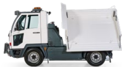
Flexible: 3-sided tipper body, e.g., for transporting bulk goods or for use on construction sites.
