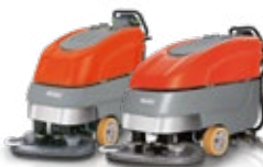
Scrubmaster B70/B90 CL Area output of up to 4,200 m²/h, 60, 65, 70, 75 or 85 cm working width
