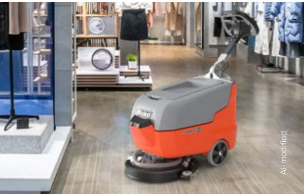
Thanks to the foldable operating handle, the Scrubmaster B25 can be folded into a compact shape for transport in the boot.
