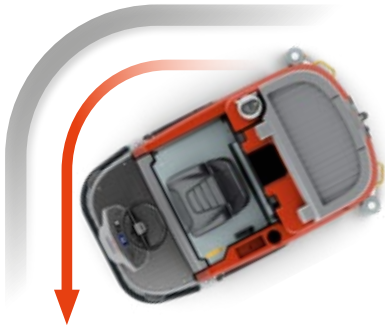
Extremely manoeuvrable The machine's 90-degree steering angle ensures a particularly small turning circle, also when working close to walls and racks.
