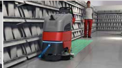
3. Automatic route calculation ensures optimised machine movement on the floor areas and aisles to be cleaned
