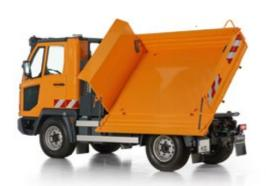
Flexible: three-way tipper with variable hydraulic tipping directions.
