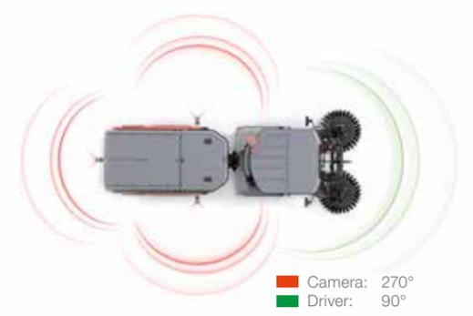
Everything at a glance: The fully glazed comfort cabin offers the driver an excellent view of his surroundings. The camera system extends the driver's field of vision by another 270° – and automatically provides a view to the side when turning.
