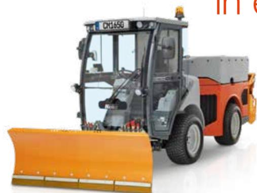
When the Citymaster 1650 is underutilised in its function as a professional sweeper due to seasonal weather conditions, the machine can be used to carry out other tasks such as grounds maintenance or winter services – which makes the Citymaster 1650 the most efficient solution for every municipal application.
