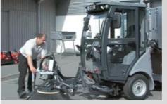
Quickly ready for use: Thanks to the quick-coupling triangle allowing easy and back-friendly changing of attachments without
