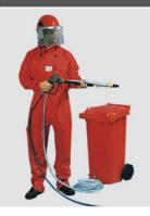
Personal protective equipment for safe, high pressure cleaning. Durable overalls made from waterproof polyamide fabric with a full-length zip and Velcro fastener – also for the arms and legs. Safety helmet with a wire mesh visor, ear protectors and goggles for enhanced safety.
