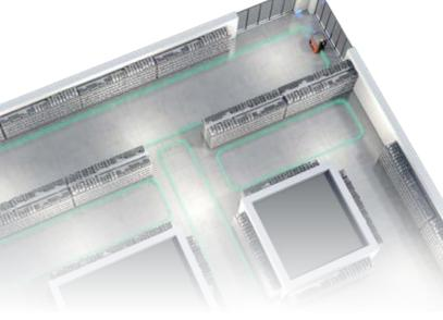
Autonomous cleaning systems follow the learned route with high repeat accuracy. This not only results in improved cleaning results, but also significantly reduces water consumption as well as the consumption of chemicals, electricity and materials.
